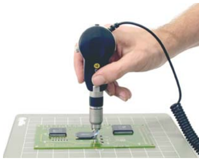
Flexia C1 ESD & Side Viewing BGA inspection Lens, free-hand operation.
